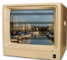
CCTV image with a ground loop problem
